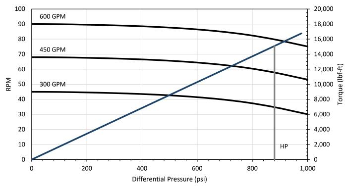
Performance curves based on testing at 70°F. Actual field performance may vary with field operation conditions.
